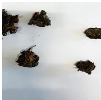
Ferromagnetic fraction of shredded WEEE" (©FAU)
